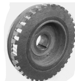
Harmonically balanced pulley - machined into trigger wheel
