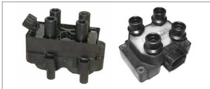
Common wasted-spark coils; Sagem / Valeo (Left) and Ford (Right)
