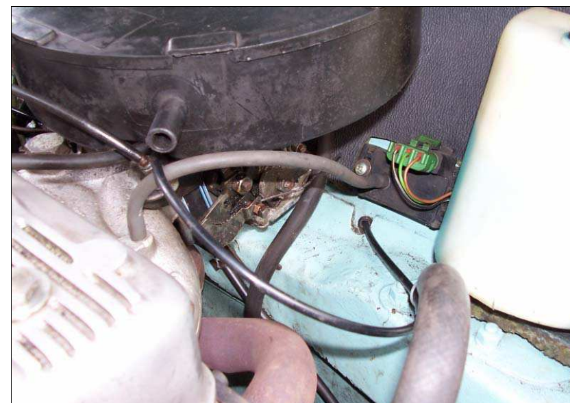
MAP sensor installed in Mini, with vacuum pipe connected to inlet manifold take-off
