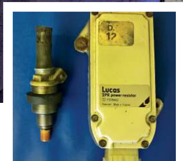
Lucas 4CU Ballast Resistor & Low Impedance Injector
